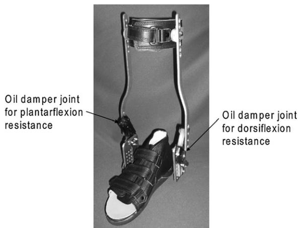
Fig. 1. Experimental ankle-foot orthosis (EAFO) [8].
